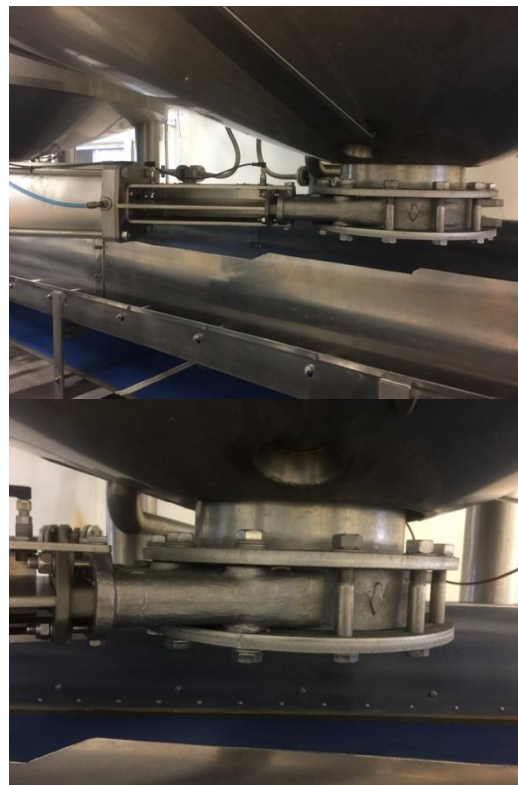
Fig. 2 Outlet valve and separations system for the enzymes.
